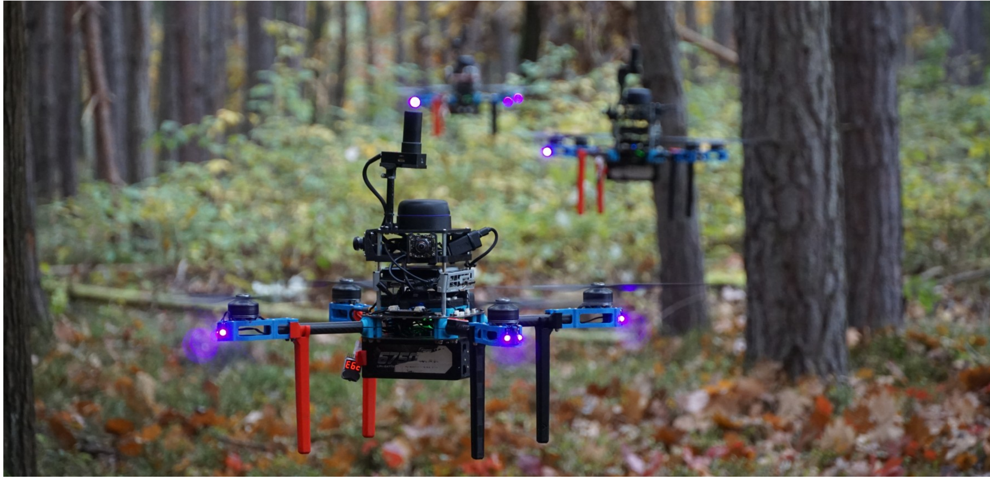
Three UAVs flocking under the forest canopy — no GNSS, no communication, only on-board sensing.
